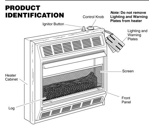
Figure 1 - Vent-Free Gas Log Propane/LP Gas Space Heater
